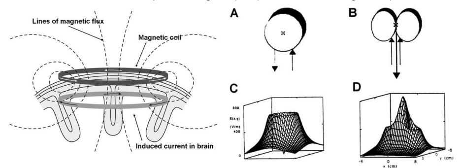
NB: field strength can be less than half strength after only ~2 cm! (Barker, 1999)
