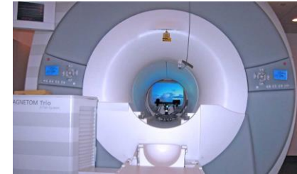
Eye tracker in MRI scanner bore: Eyelink 1000 - SR Research
