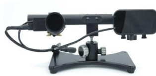
Eye tracker in MRI scanner bore: Eyelink 1000 - SR Research
