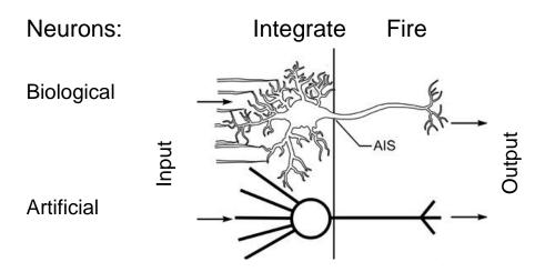
Integrate-and fire neurons: multiple dendrites and one cell body (soma) receive and integrate synaptic inputs as membrane potentials which are compared to a threshold at the axon initiation segment. If threshold is met, axonal spikes/firings are triggered along a single axon which branches distally to convey outputs.
